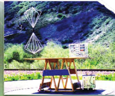
Open Air EMI Emission Testing to CSPP 22
