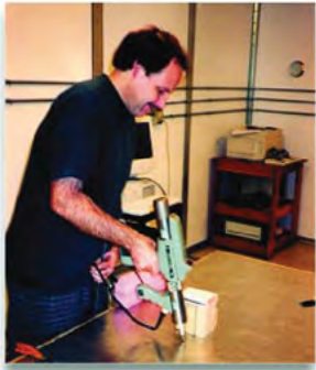
ESD Testing ±2KV,4KV,8KV & 25KV
