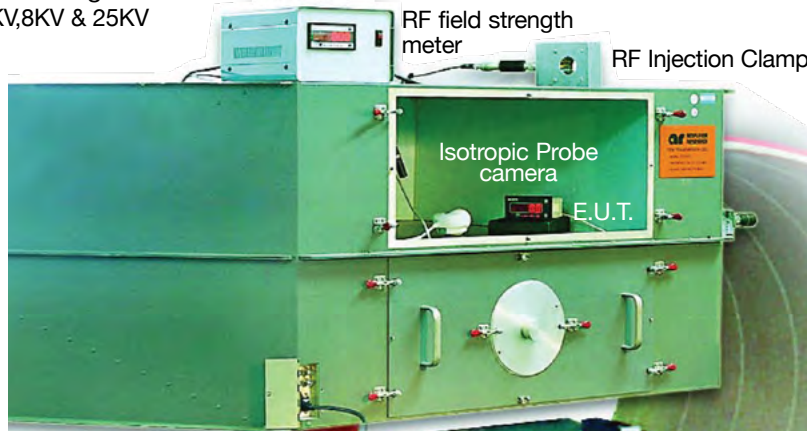
Laboratory TEM Cell for testing RF Immunity and Emissions RF inputs from 50 to 500 MHz at field strengths up to 300V/m. Completely shielded from external noise, precision RF emissions can be measured, from 30 MHz to 1 GHz at 10 to 500 dB-microvolts.
