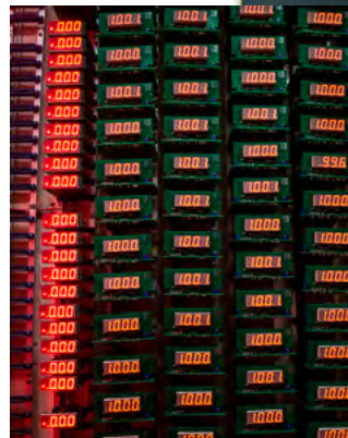
Life Testing at elevated temperatures
